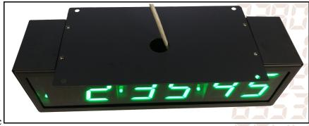
plug is typically placed into the side hole of the clock and all wiring connections are done through the top hole. In the case of a WiFi clock, the WiFi antenna can be placed above the ceiling for a completely hidden installation.
