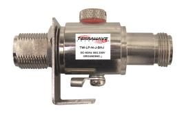
Ventev's TerraWave Lightning Arrestor is a bi-directional gas discharge tube suppressor that features wide-band operation up to 6 GHz and is rated at IP67. Simply attach the lightning protector to an access point to help protect an entire network, outdoor antennas and other wireless equipment from the build-up of static electricity. It is recommended to use 18 American Wire Gauge (AWG) ground wire.
