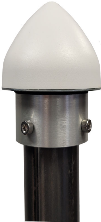
Collar Mount: Goes on Top of up to 1.5" OD pole. Held in place with two set screws. Cable is contained inside of pole.
