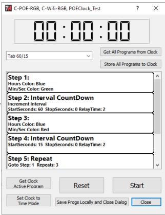
If a clock is executing a timer program when the dialog is opened, it will update and display the current state of that timer program, joining the program in real-time. Perfect synchronization is not achieved, but close.
