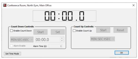
allowing control of separate clocks with separate count up/down parameters. The top of the dialog box window will list the names of the clocks being controlled. Those clocks will be grayed out in the main window such that they cannot be selected for control in a second window at the same time.
