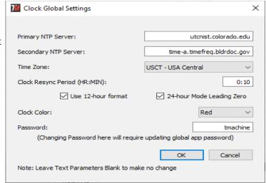
The parameters will be updated to each selected device when OK is clicked. A progress meter will be displayed on the main window during the update process.
